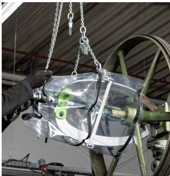
Safety cover guarantees a secure removal
