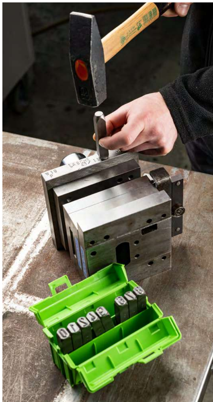
Marking a punching tool with impact numbers of series 328
