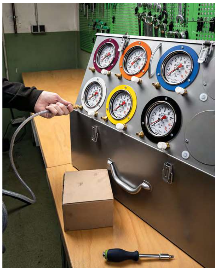
Connecting a pneumatic hose to the coupling socket
