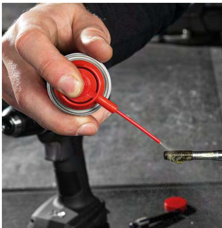
Greasing the thread
