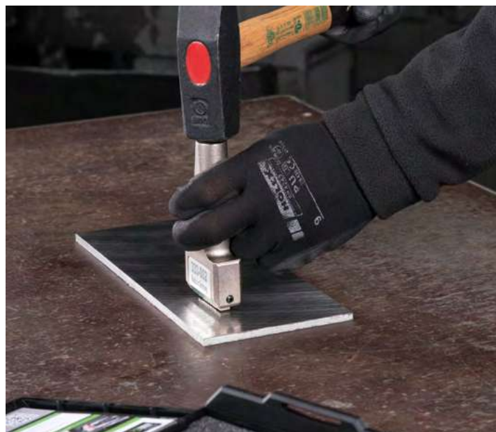
Marking a steel plate with a punch stamp from series 333
