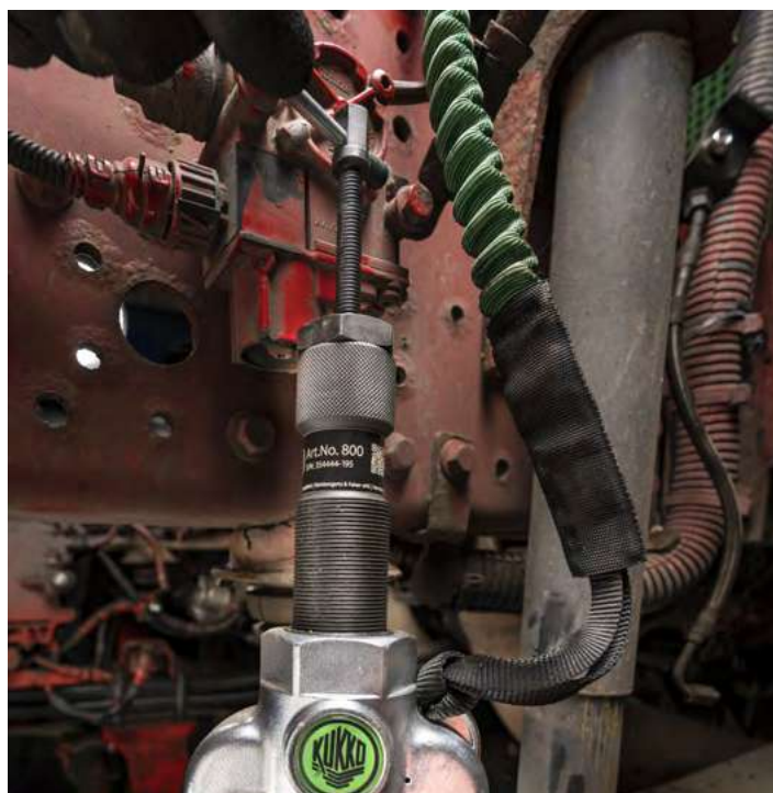
Safety puller secures ball joint puller
