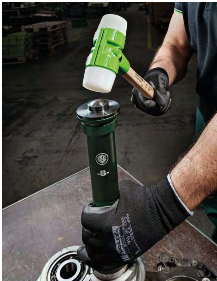
Installation of a bearing with a soft-face hammer Selecthor in combination with the 71-L
