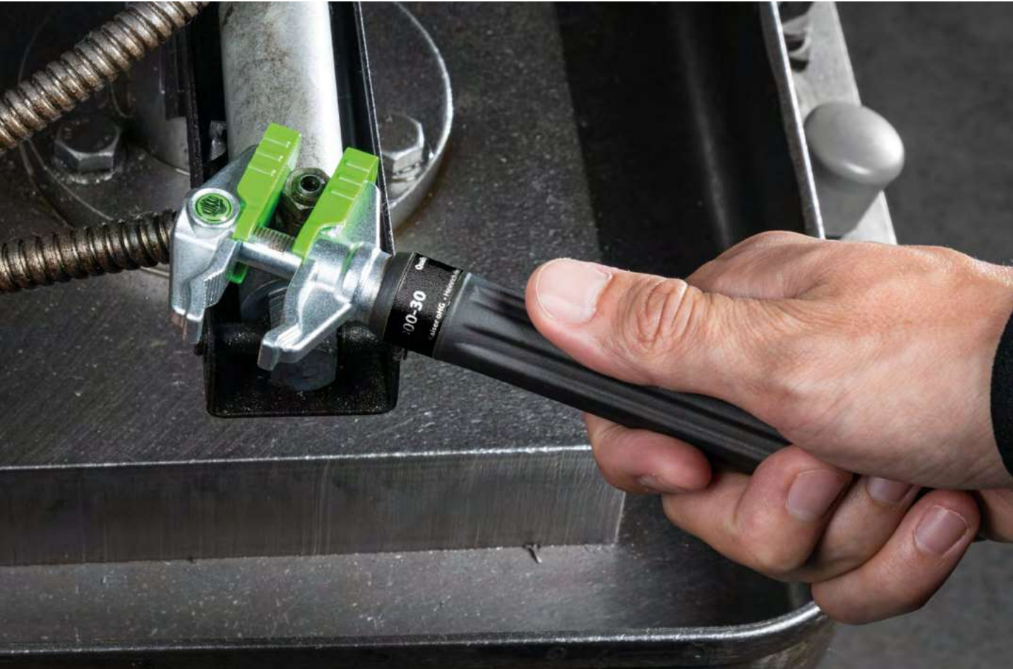
Loosening a nut with the European 1900-30.
