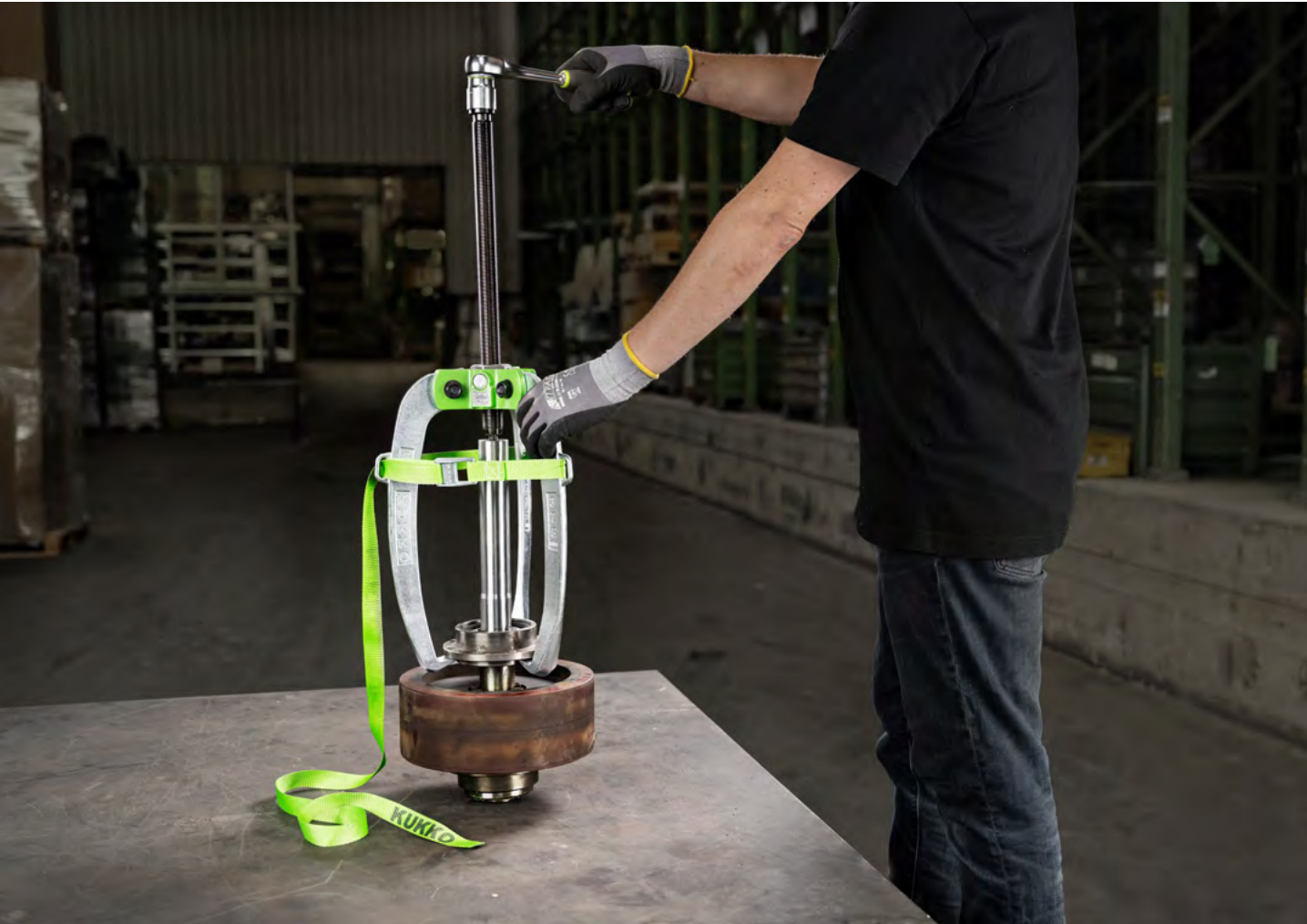
The USB-1 tensioning strap secures a 3-armed industrial puller during pulling
