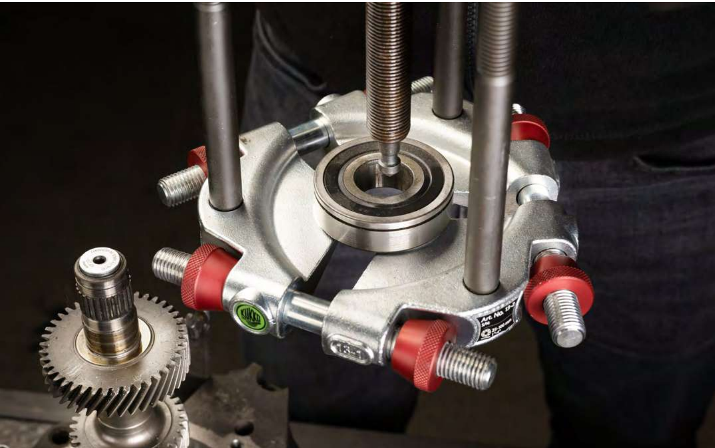
The three-part TRI-PULL 13-2 separating device when removing a seized ball bearing
