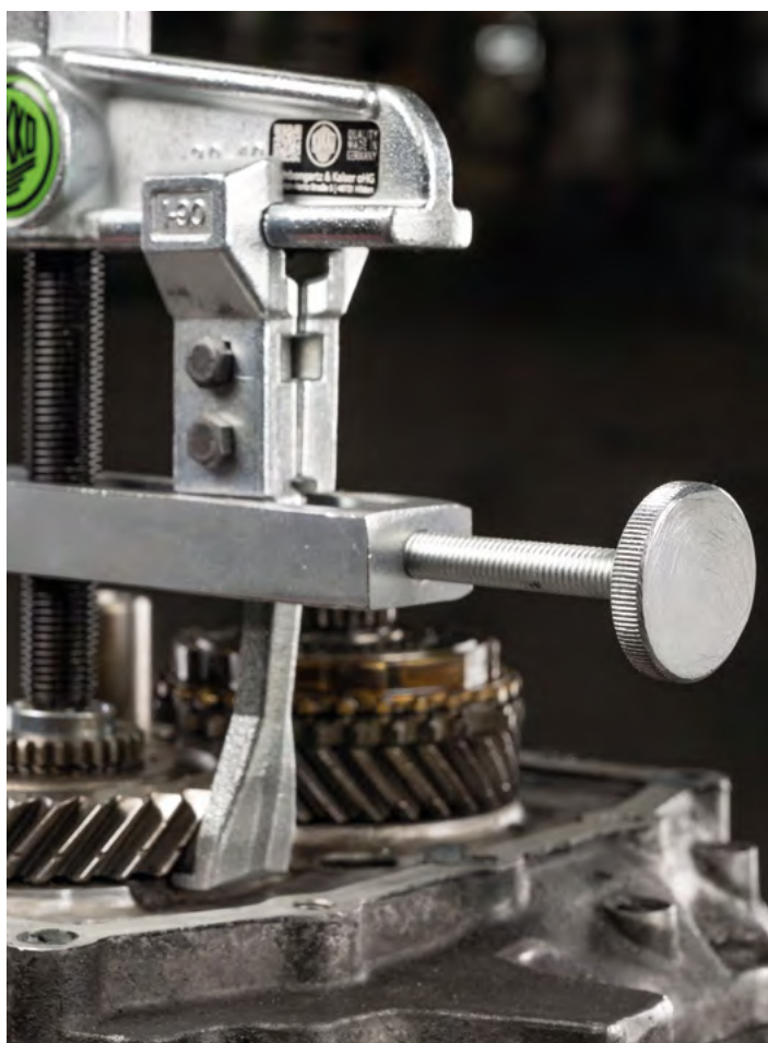
The clamp presses the arms against the part to be removed.
