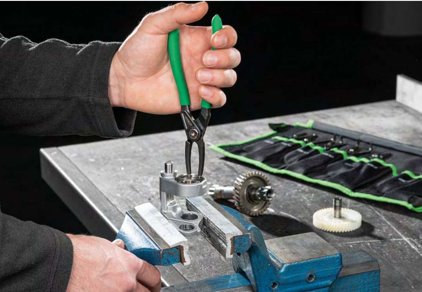
A pair of pliers from the circlip pliers set 728K-729 is used to remove a stuck circlip
