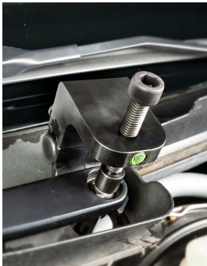
Removing a wiper arm with the 128-F-60
