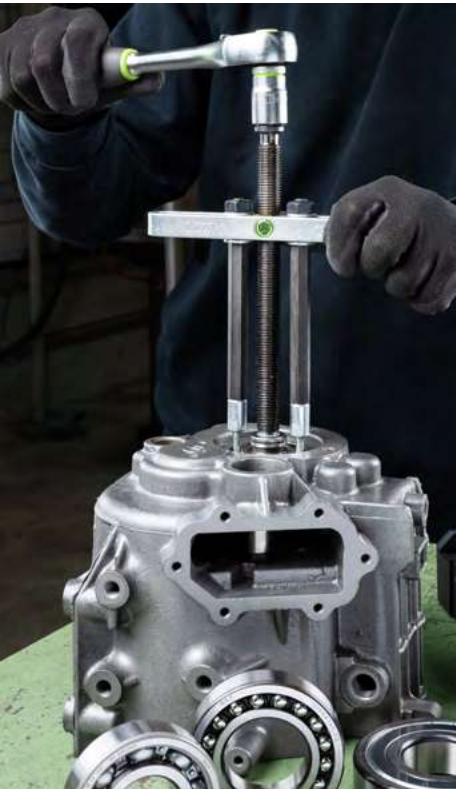
Ball bearing disassembly with the 69-A
