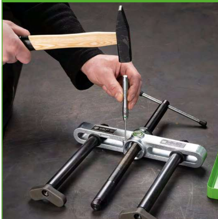
Driving out a retaining pin with a pin punch
