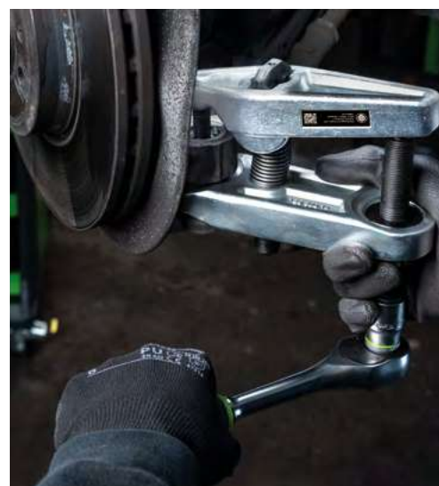
The spherical joint puller 129-3 when pressing out a tie rod end in a workshop
