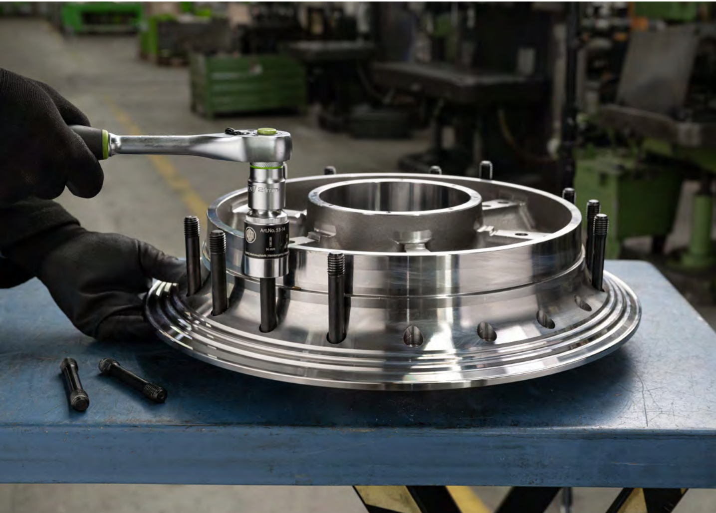
Removing a gear with the 47-1-A
