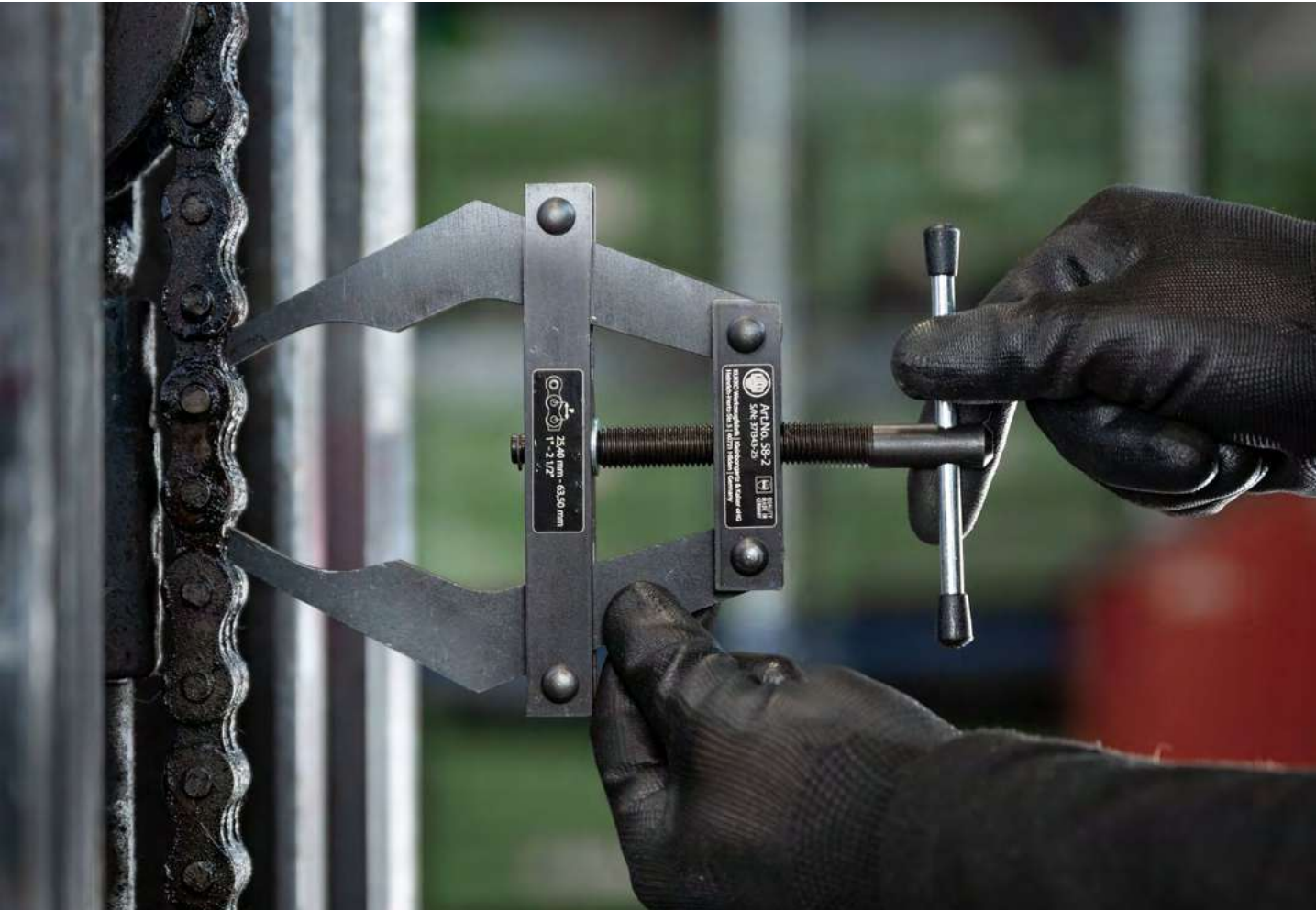
The 58-2 assembly tensioner is used to tension the lift chain of a forklift truck to make it easier to dismantle
