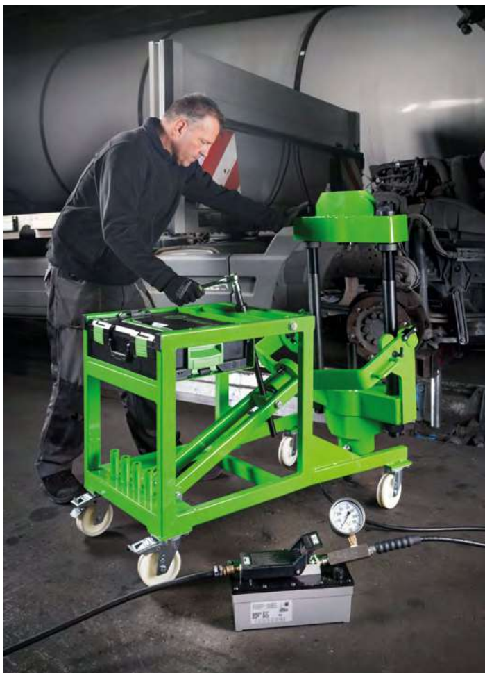
The hydraulic axle joint bolt press "AXLE" Y-AP-75 is adjusted with a ratchet.
