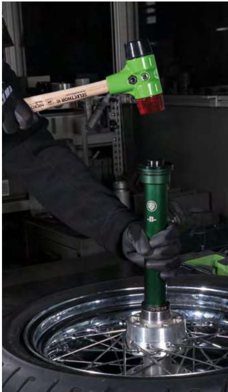
Bearing installation with the 71-L
