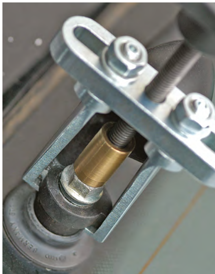
Removing a wiper arm with the 128-F-SW
