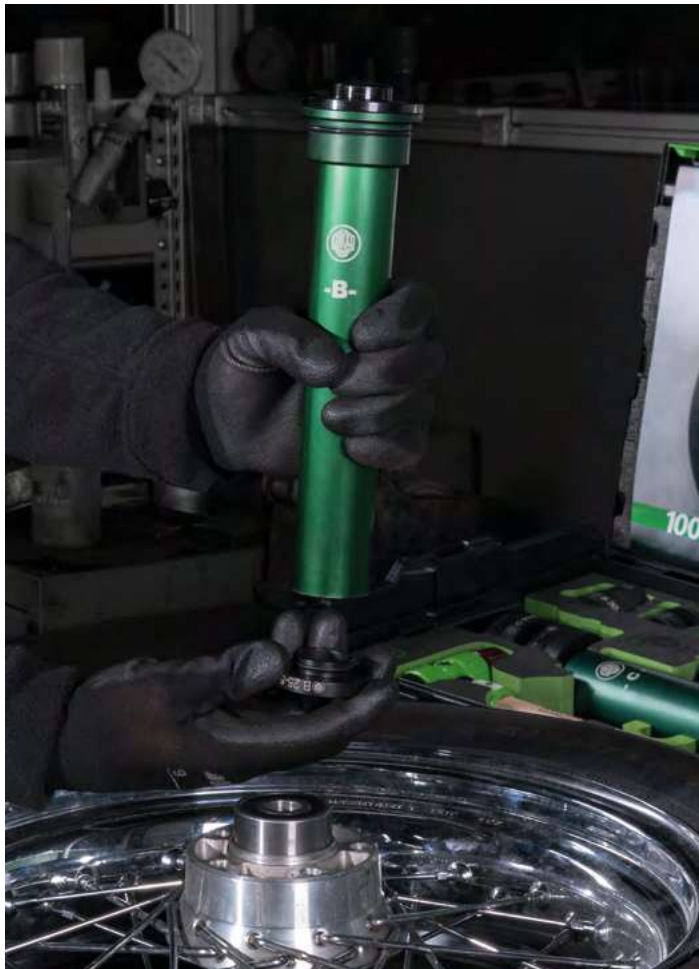
Inserting the appropriate impact ring into the impact tube when using a K-71 set
