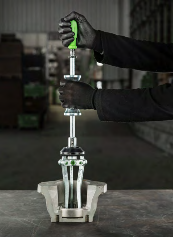
Internal extraction of a ball bearing from a housing
