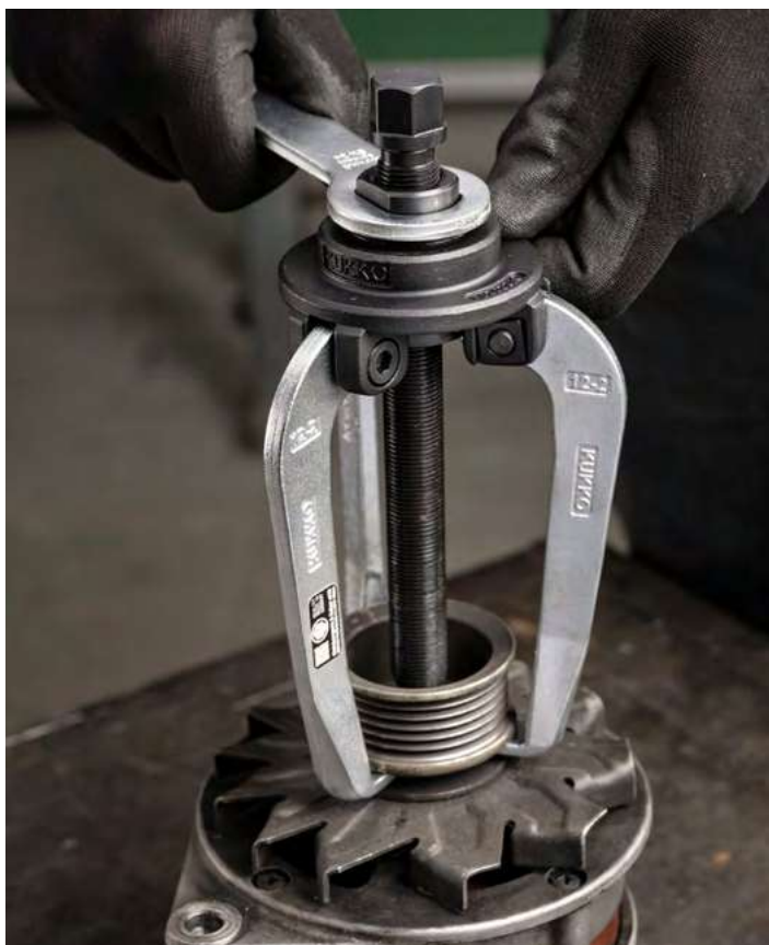
Removing a pulley from a car generator
