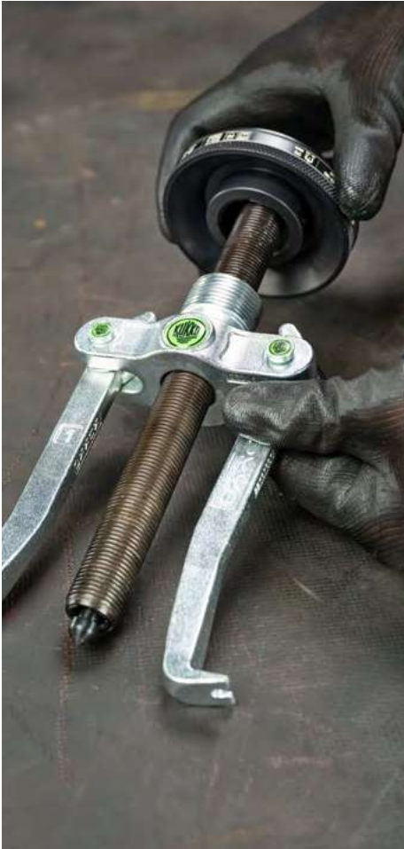
Mounting the clamping cone rotated by 180°
