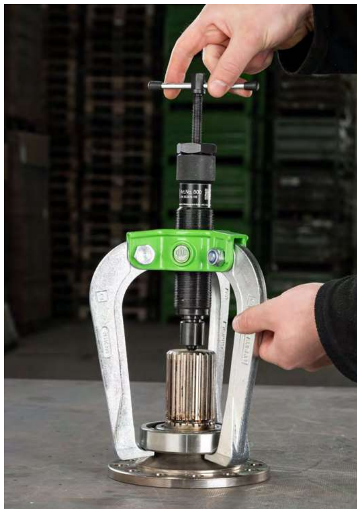
Actuation of the T-handle for the construction of hydraulic power
