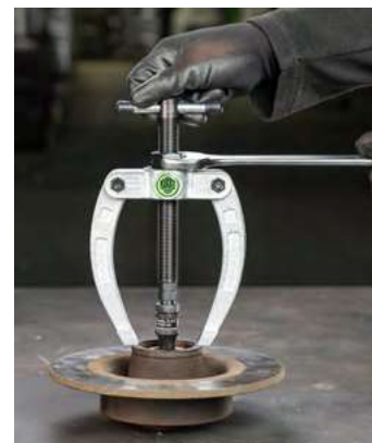
Internal extractor with counter stay
