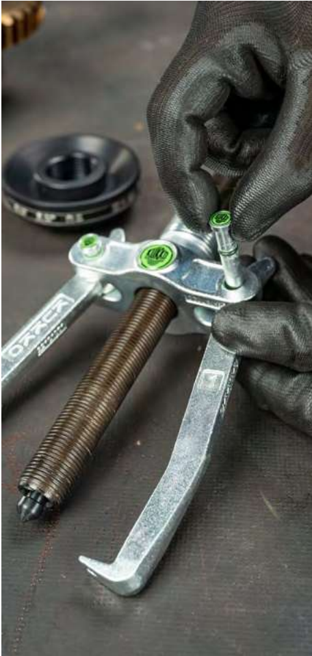
Removing the socket pins
