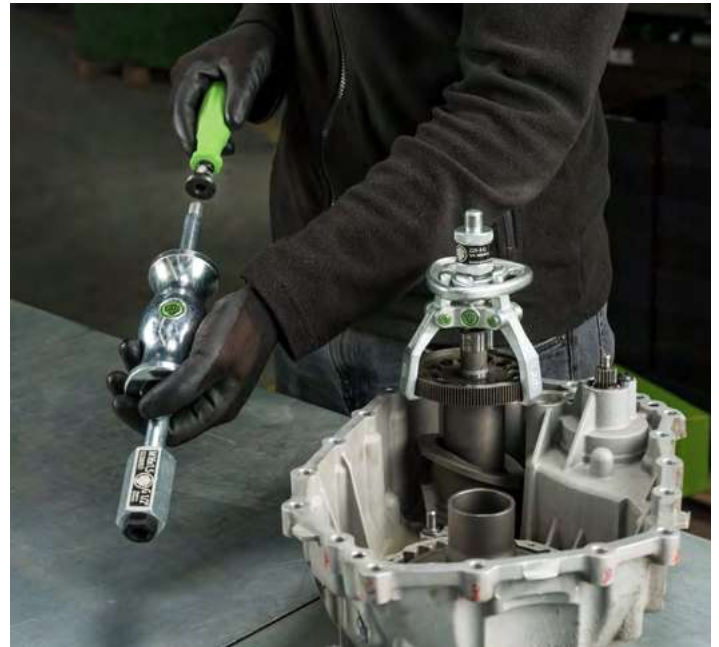
Attaching the 3-K grip G-22 to the sliding hammer
