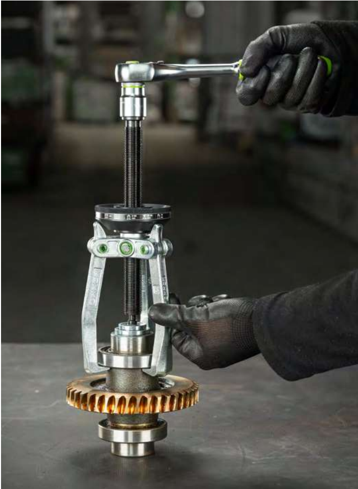
External removal of a ball bearing from a gear shaft
