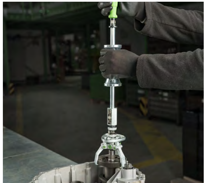
Dismantling a pulley from a transmission part
