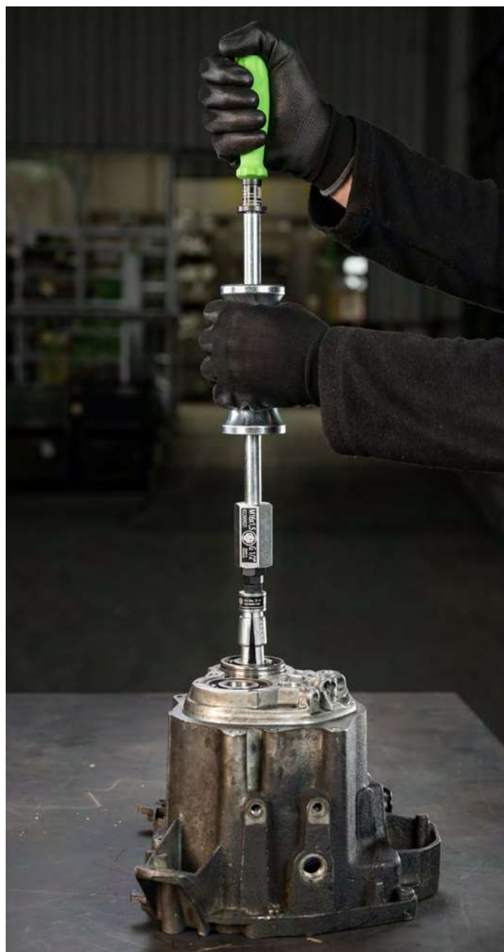
Internal extraction of a ball bearing with the 21-4 and a sliding hammer
