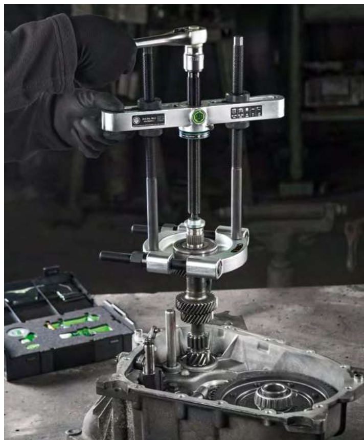
Removing a bearing from a gear shaft
