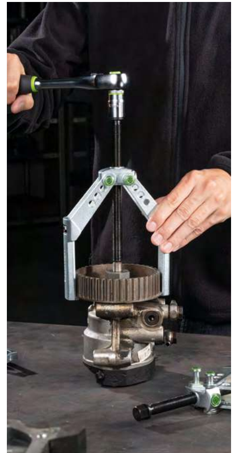
The uncrossing of the puller jaws greatly increases the span range.
