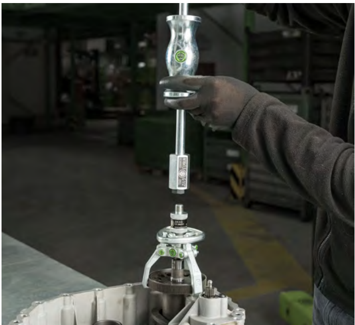
Connecting the sliding hammer via the thread adapter of the puller
