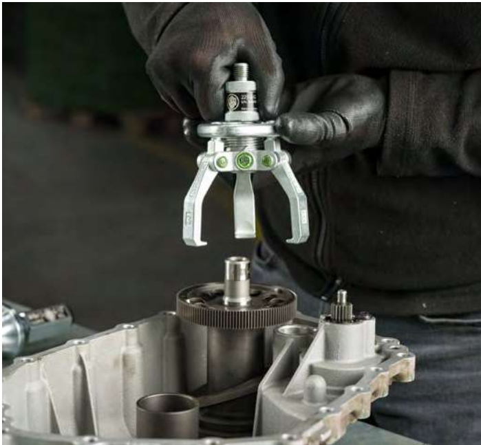
Setting the puller on the part to be pulled off
