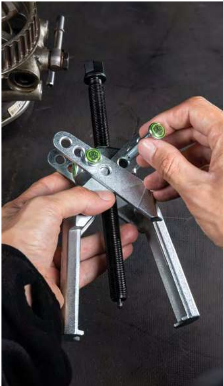
Manually removable locking pins
