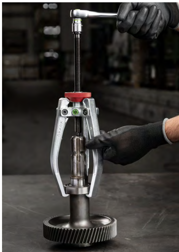
The 3-jaw puller 113-3 with cone knob when extracting a ball bearing from a gearbox
