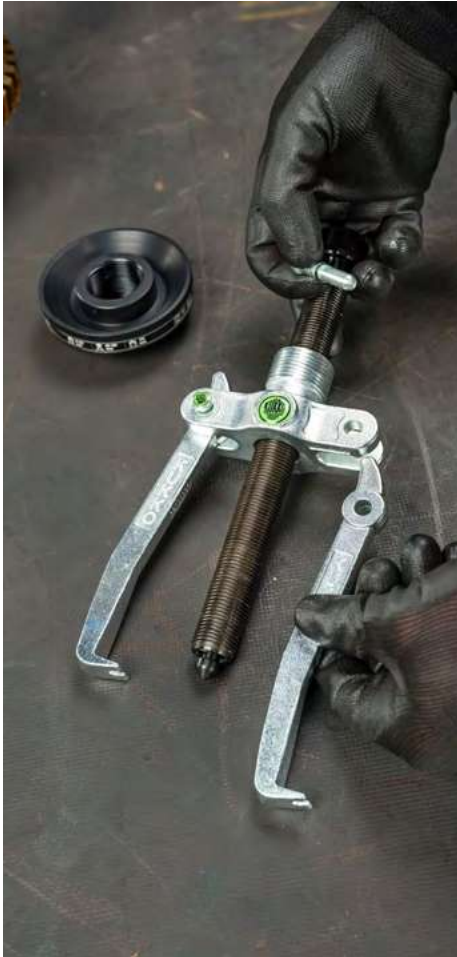
Turning the puller legs
