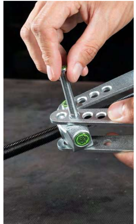
The legs are adjusted and the locking pin is inserted.
