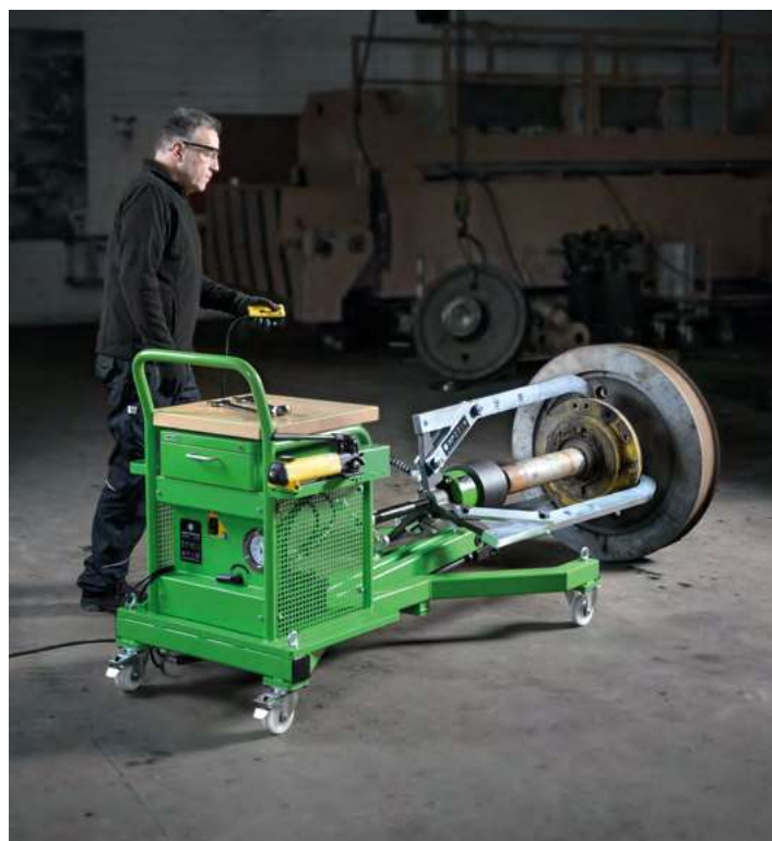
The mobile hydraulic puller "GOLIATH" Goliath-556 when removing a stuck wheel bearing from a harbor crane.
