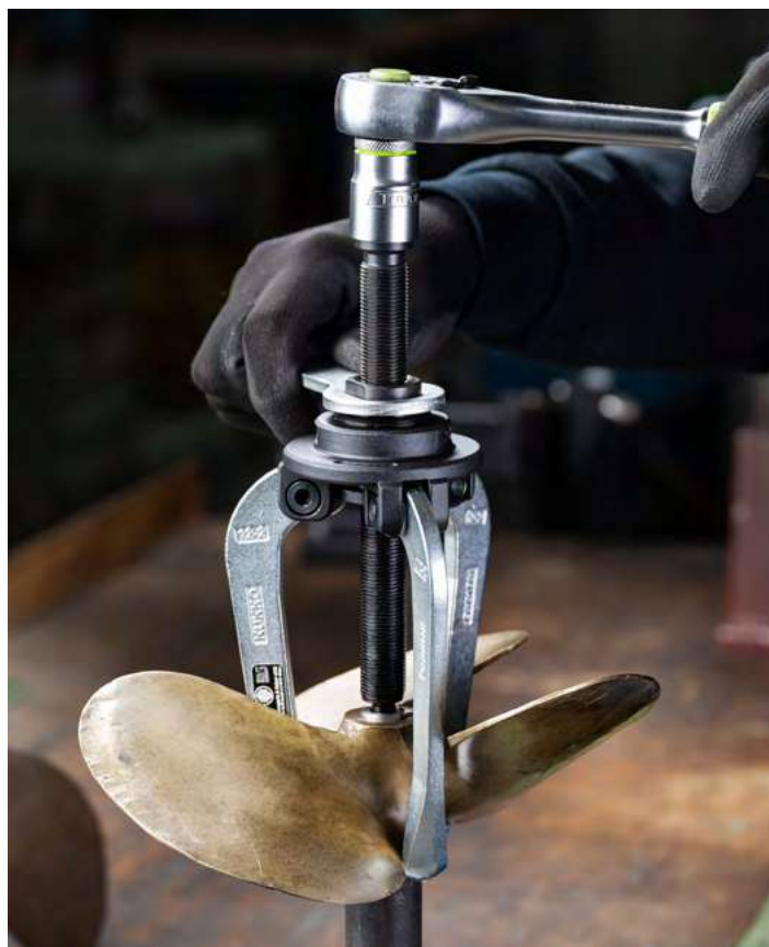
Dismantling a ship propeller with the 12-2
