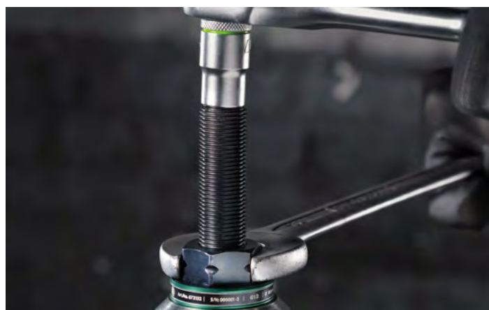
The Power Nut reduces the effort required to actuate the spindle.
