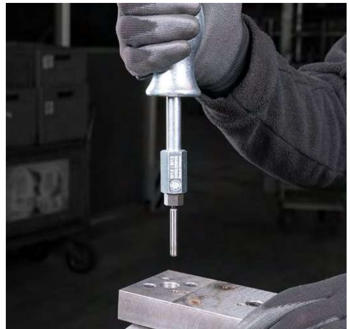
Removing a dowel pin using a sliding hammer and thread adapter
