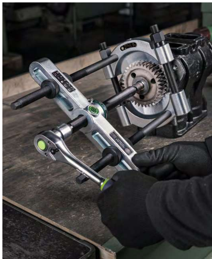
Removing a gearbox gear
