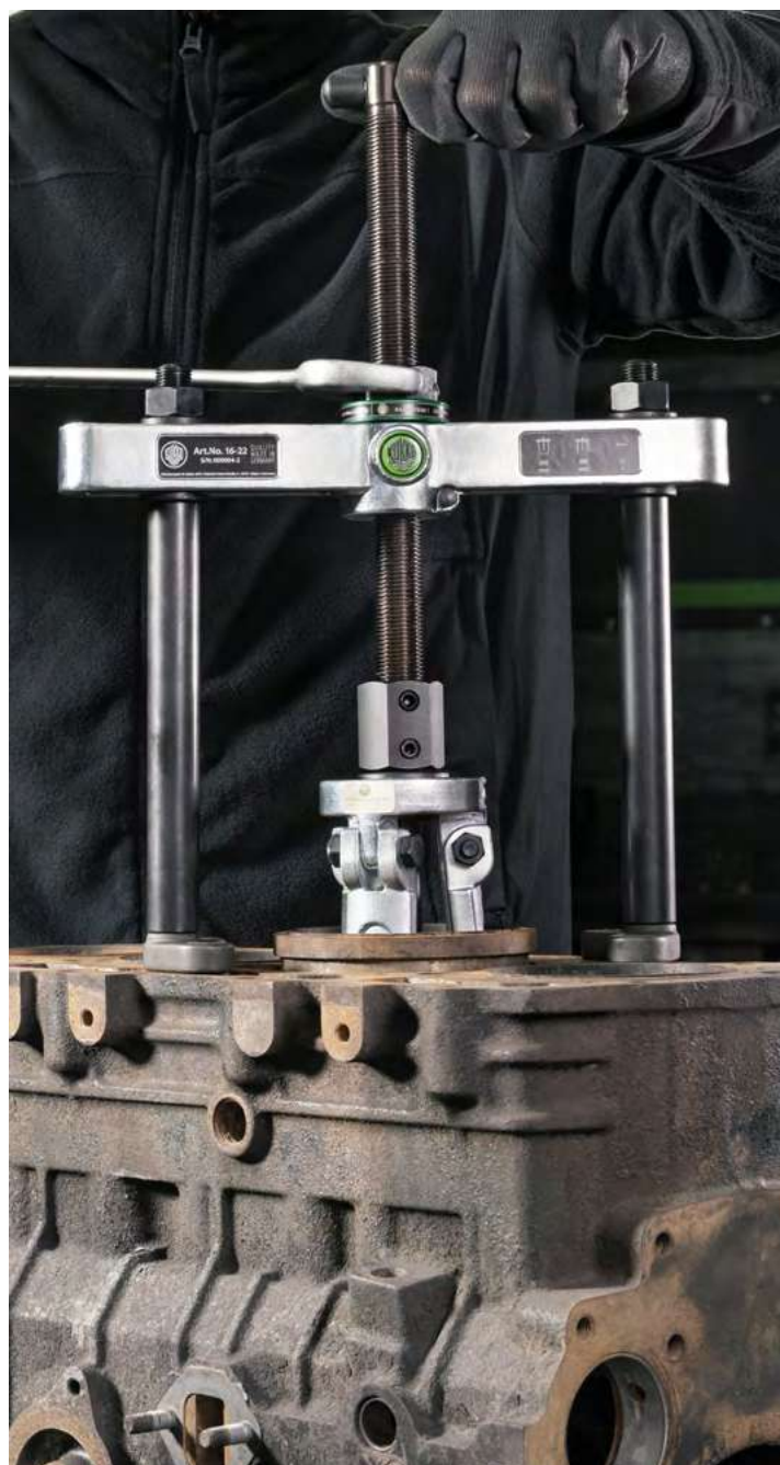
Removing a cylinder sleeve with the 21-90 and the counter stay 22-5
