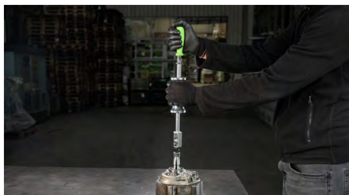
Removing a ball bearing with a sliding hammer and an internal extractor from series 21
