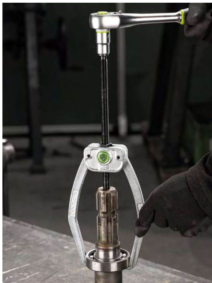
Dismantling of a ball bearing from a gear wheel
