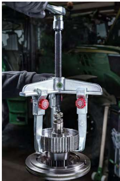
Removing a gear from a shaft with the 30-10+
