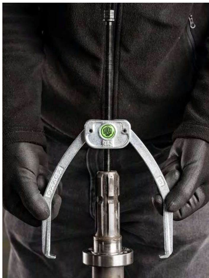
Positioning the puller jaws on the component to be disassembled
