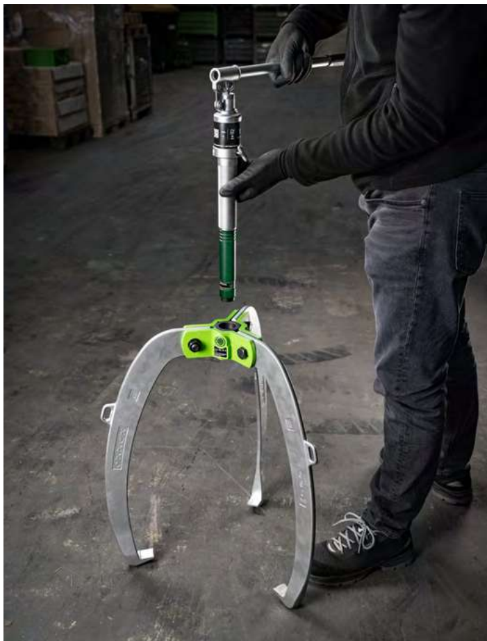
Inserting the hydraulic spindle
