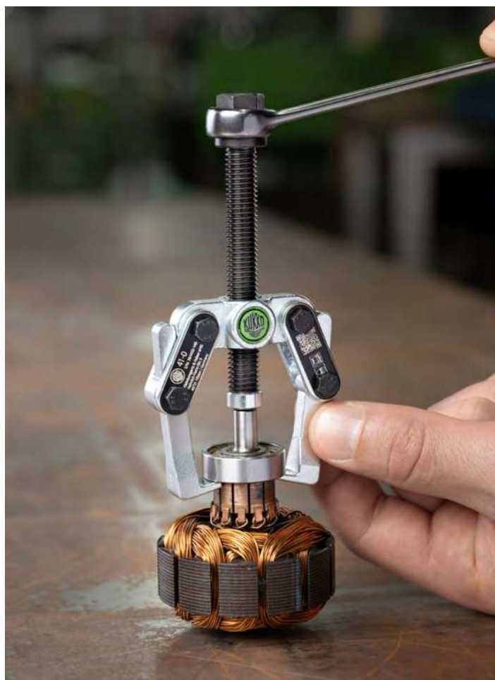
Removing a small ball bearing from an E-motor shaft with the 41-0
