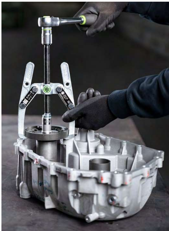
Expansion of a gear wheel with the 205-01
