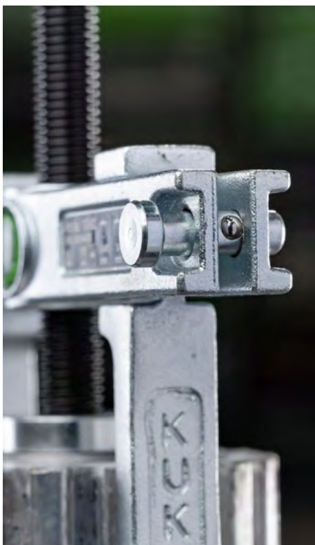
The spring-loaded ball secures the pin against slipping out.
