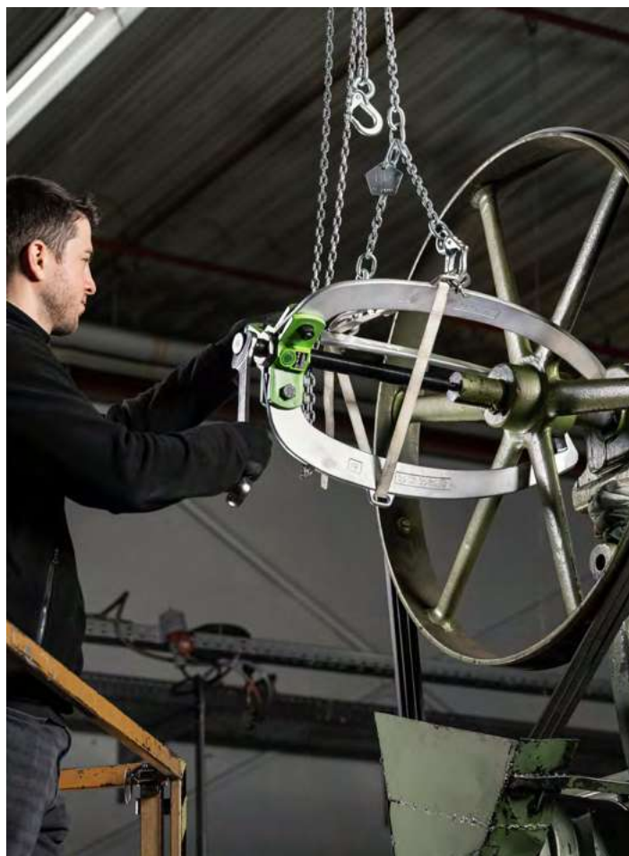
An additional tension belt secures the jaws
