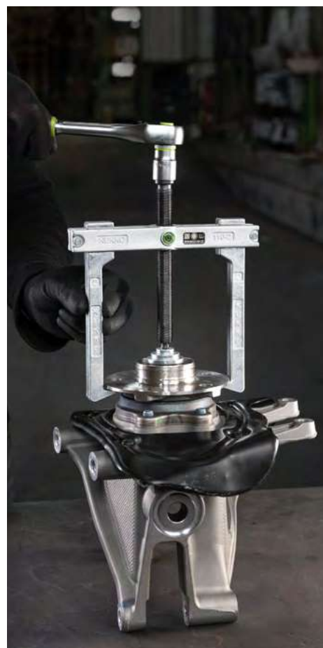
Removing a hub from a steering knuckle with the 110-2
