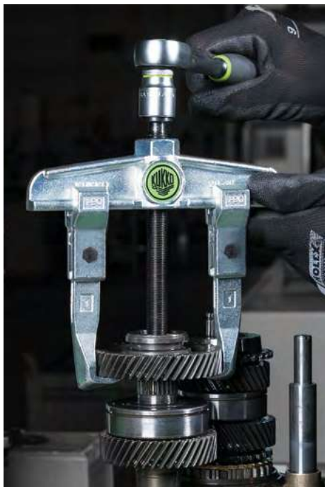
Removing a gear wheel with the 20-10
