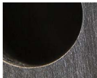
After machining - Burrs have been reliably removed and the edges rounded. The surface has a uniform, brushed appearance.
